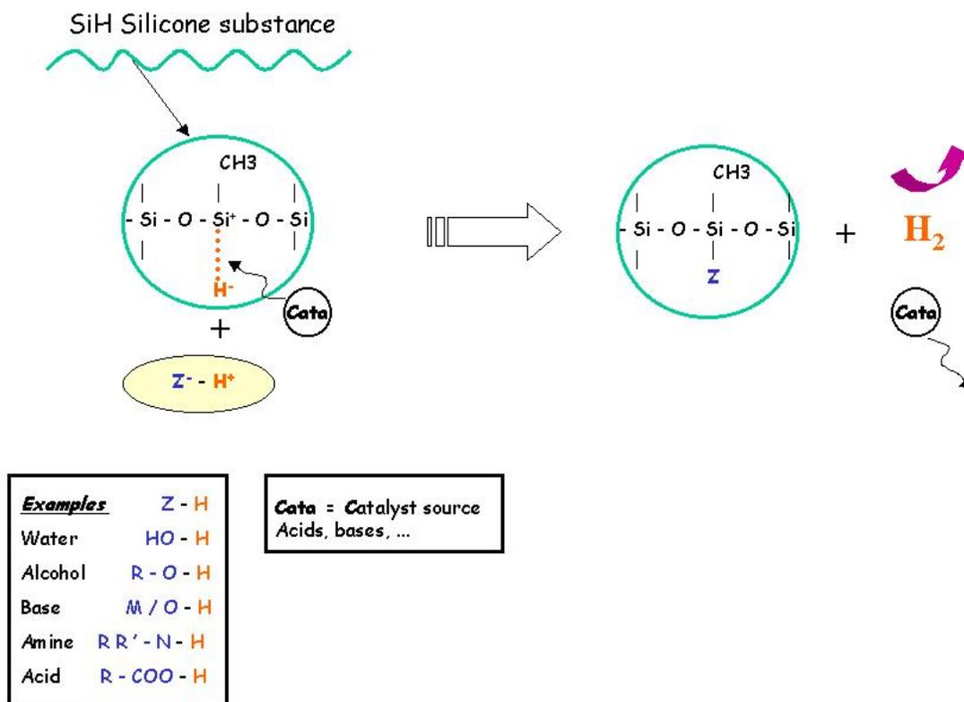
FIG. 1—Gassing Phenomenon of SiH Products.
